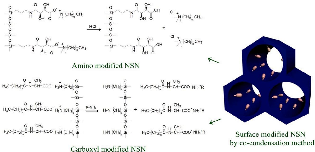
Fig. 2. Formation mechanism of surface modified NSNs with co-condensation method.
