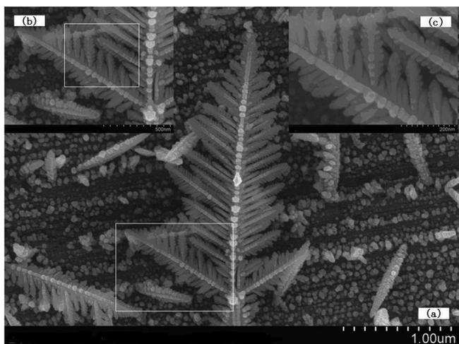
**Fig. 1.** SEM images of silver dendritic nanostructures on copper foil: (a) The whole structure (b) The structure of side branch (c) The structure of the secondary side branch.
