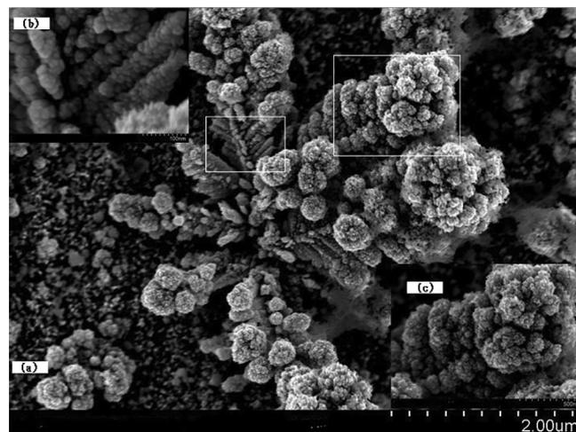
**Fig. 3.** SEM images of silver nanostructures on tin foil: (a) The whole structure; (b) The bottom structure of the branch; (c) The top structure of the branch.
