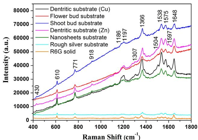
Fig. 5. Raman spectra of R6G solution on different SERS substrates and R6G solid.
