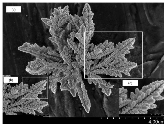
**Fig. 4.** SEM image of silver nanostructures on aluminum foil: (a) The whole structure (b) The structure of side branch (c) The structure of the secondary side branch.
